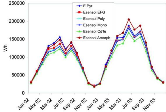
Figure 4: Monthly solar energy measured in-plane of the solar modules for the years 2002 and 2003. The solar irradiance was measured with a standard pyranometer and with Sensol® with different cell technologies.
