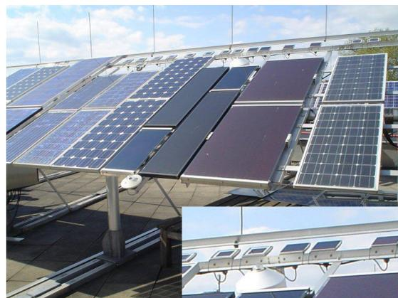
Figure 1: Setup for the long term monitoring of PV modules on a rack with fixed position. Solar radiation is measured with pyranometers and with Sensol®. For each module technology a Sensol® with corresponding cell technology is available (see detail).
