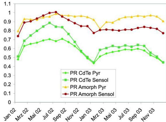
Figure 8: Monthly performance ratio PR for PV modules with thin film technology. The performance ratio was evaluated with radiation data measured with either pyranometer or with Sensol® with corresponding cell technology.
