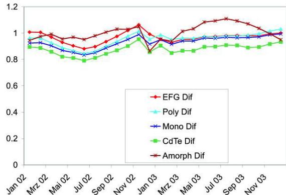
Figure 5: Signal of Sensol® relative to Pyranometer.
