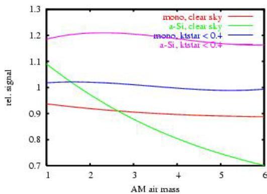
Figure 3: Variation of Sensol® signal relative to pyranometer as function of air mass AM for clear sky conditions ( $k_t^* > 0.8$ ) and overcast conditions ( $k_t^* < 0.4$ )
