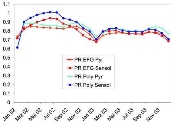
Figure 7: Monthly performance ratio PR for PV modules with crystalline cells. The performance ratio was evaluated with radiation data measured with either pyranometer or with Sensol® with corresponding cell technology.
