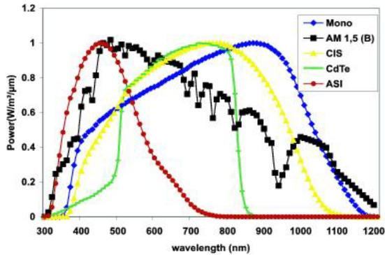
Figure 2: Spectral sensitivity curves of solar sensors Sensol®.
