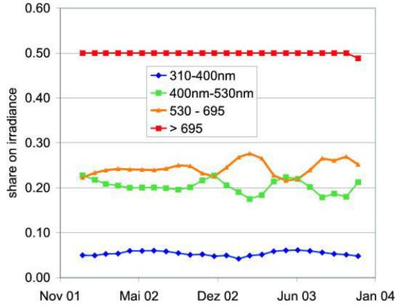
Figure 6: Share of selected spectral bands to the monthly solar irradiance. Data are measured with pyranometer equipped with filter and a UV-A pyranometer.
